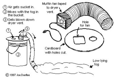
into the water the heavy fog is generated and blown down the hose. These "Big boy" versions are really what is needed to give good ground coverage over a large area.
